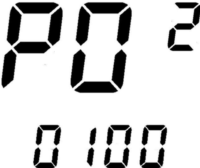
The P02 parameter is used to correct the currently displayed speed value. This parameter works regardless of the phase voltage speed or the Hall speed. The purpose is to correct the current speed display value. The coefficient value is between 0.20-1.50 (actual display 20-150), each time the button jumps the value 5, the actual corresponds to 0.05, the value changes as follows: 10->15->20->....100->105-> 110->....->150->10
