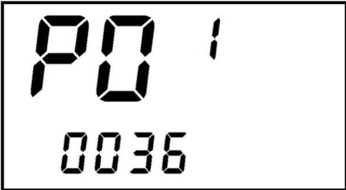
When the lower number is flashing, press the button to select the actual value of each parameter:
