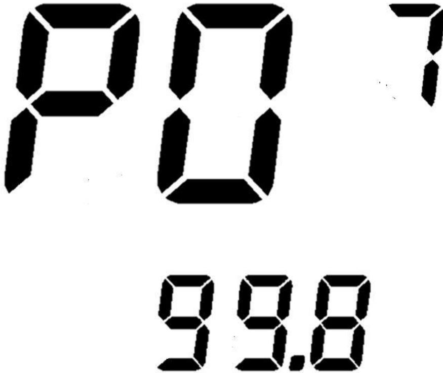
This parameter is similar to the speed coefficient. The customer feedback battery voltage measurement value is not accurate. This parameter is used to correct the battery voltage value. The value of this parameter is from 95.0% to 105.0%, and each press of the button increases 0.2%.
