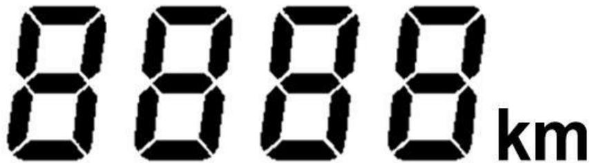
After entering the P09 parameter, press and hold the (>3 seconds) button to accumulate the mileage. At this time, press the button 10 times continuously to clear the accumulated mileage.
